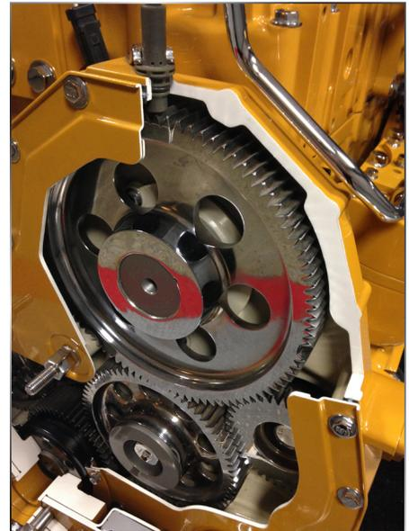
Crank and cam gears are easily installed and removed
