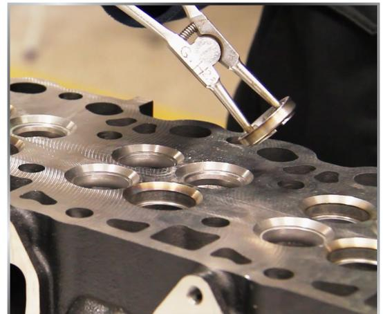
Cooled valve seat ring contracts, allowing easy removal
