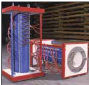
Titanium billet-heating coils for extrusion process
