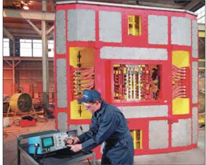
Reconditioning, overhaul and replacement of ladle stirring units
