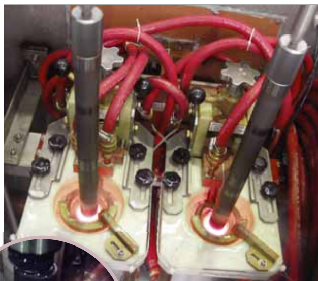
Quick change inductor tooling and enhancements to quench are available for all heat treating applications.
