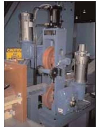
Pinch roll drive
