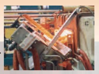
■ 150 kW, 10 kHz automatic bar end heater on a unitized base, with drop bottom tote box loading.
