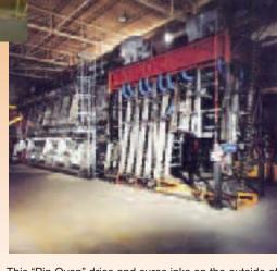
This "Pin Oven" dries and cures inks on the outside of beverage cans. Typical speeds of these ovens are 2000 cans per minute.
