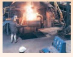
▼ This 90 ton vertical channel furnace increased gray iron pouring capacity without increasing energy cost during peak demand periods. It acts as a buffer between primary melting and molding requirements providing a continuous flow of temperature-controlled and metallurgical constant iron.
