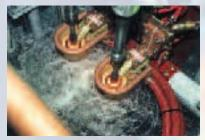
Yoke shafts and flanged axles are induction hardened and tempered at rates up to 50 parts per hour on dual spindle scanners. Scan speeds and power levels are precisely controlled and monitored with servo drives and computer operator interfaces.
