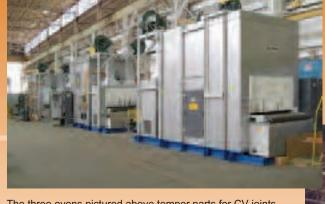
The three ovens pictured above temper parts for CV joints on front wheel drive vehicles. In each oven 240 parts per hour are heated to 450 degrees F for one hour, then cooled to room temperature in less than 20 minutes.
