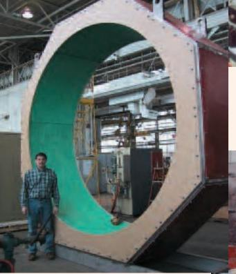
Nine megawatts of power is used to preheat tubing for stretch reducing. Induction heating advantages include fast start and stop capabilities, low scale formation, better surface quality, speed and scheduling flexibility.
