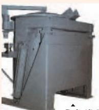
The Steel Shell Furnace design provides maximum strength and support for all melting applications. Ideal for use with charge buckets and vibratory conveyor charge systems.
