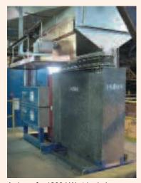
A view of a 1200 kW strip drying application. This equipment is being used for a wide variety of coating applications. The equipment is designed for horizontal or vertical installations.
