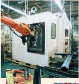
Robots load and unload heavy truck axle tube assemblies into a heavy duty single spindle vertical scanner for hardening and tempering.
