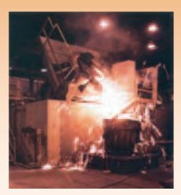
Two 3600 kW medium frequency solid state power supplies are used here with two 10 ton coreless furnaces to provide this foundry with the flexibility required to meet a variety of hot metal needs. The ruggedness of the Ajax TOCCO design provides day in and day out trouble-free operation.
