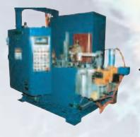
Factory cell and pick and place systems such as this Ajax TOCCO designed hub hardening unit are completely self-contained and shipped ready for utility hook up. They are ideal for achieving consistent high quality and reducing labor costs.
