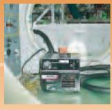
A 5kW TOCCOtron AC power source is shown within the confines of a NASA space shuttle. This 100% air-cooled system is used to braze critical fuel and hydraulic lines. Its lightweight and small size allow it to be placed most anywhere within the orbiter.
