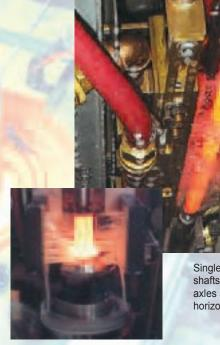
Stems of CV joint components and wheel spindles are hardened on a variety of standard and custom designed lift and rotate systems. Single shot hardening of drive shafts, transmission shafts and axles are provided utilizing horizontal and vertical systems.
