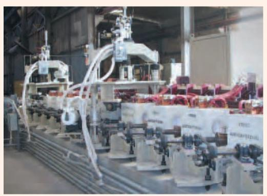
Ajax TOCCO quench and temper lines for solid bars and shapes are known industry wide for producing superior metallurgical and physical properties in the final product. These benefits are achieved with the ultra high heating rates and temperature control possible only with induction heating.
