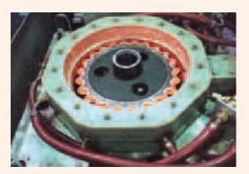
Dual frequency heating of sprockets provides uniform root and tip temperatures required for hardening. The programmable lift fixture is designed to harden sprockets up to 25" diameter using up to 1000 kW.
