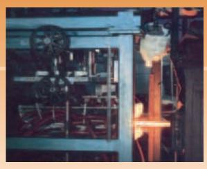
Ajax TOCCO, Transverse Flux heating is changing the way processors want to heat strip. TFIH enables the user to heat a wide variety of strip with the same inductor and enables our customers to make adjustments to the system without shutting down the line. Processing costs can be cut as much as 22%, and scale formation reduced as much as 67%.
