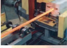
Sway bars for automobile suspensions are forged with this Ajax TOCCO heater. Bars are continuously fed through five cast coils for fast scale free heating.
