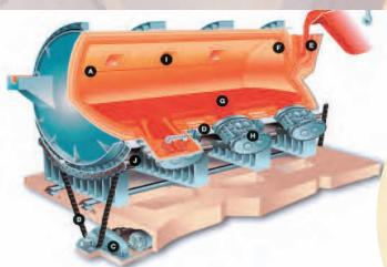
Ajax TOCCO leads the industry with high powered Jet Flow channel inductor technology. This, coupled with our innovative large furnace designs, has allowed us to create "Superheaters" for the steel industry. Superheaters are designed to melt scrap and superheat blast furnace iron prior to introduction into a steel making process. Ajax TOCCO designs and manufactures the world's largest channel induction furnaces.
