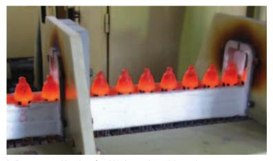
In-line automated brazing of carbide inserts into mining tools
