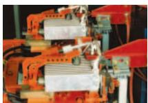
Aluminum brazing of tube-to-tube connections
