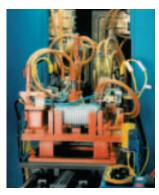
Single station manual brazing of aluminum evaporator cores
