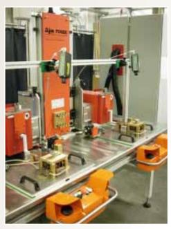
Integrated dual station system with optical pyrometer sensing
