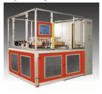
Utilizing the modular concept of the single and dual station universal brazing system, the rotary dial allows for even greater production capabilities. Beyond the operator loading station, the first cassette is under power and brazing while the successive stations are used for continuous gas cooling of the parts preventing oxidation.
