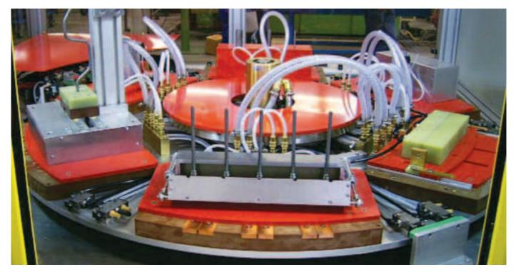
System utilizes a variety of brazing fixtures to produce continuous or mixed production. The process tooling identification with stored process parameters are programmed and identified in each tooling cassette.
