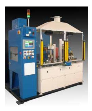
Unitized Dual Station Brazing System with integrated part program storage, illuminated working area and quick change tooling
