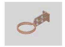
Helical Coil (encircling)
