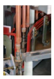
Rotary indexing soldering system featuring all stainless steel construction, alloy wire feeder and designed for high-volume production of non-ferrous tube and fitting assemblies.
