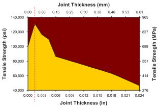
Optimal Fill Gap (Heated Parts)
