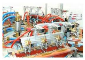
Independently controlled power supplies with braze tooling designed with chambers providing atmosphere cover of pure Nitrogen or Nitrogen/Hydrogen mixture
