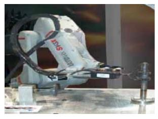
Adaptable robot configurations for "in-place" brazing
