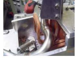
High temperature copper brazing of stainless to stainless tube assemblies in a shield gas fixture
