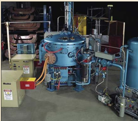
Multi-stage vacuum/atmospheric controlled system for induction preheat/melting/infiltration using internal robotics for part transfer
