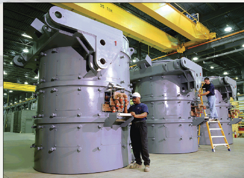
25 ton vacuum furnaces incorporate "HPD" coil designs.
