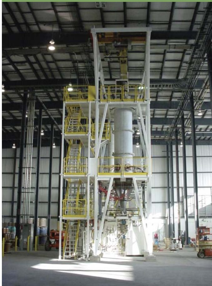
Typical continuous vertical multizone induction heating and cooling reactor
