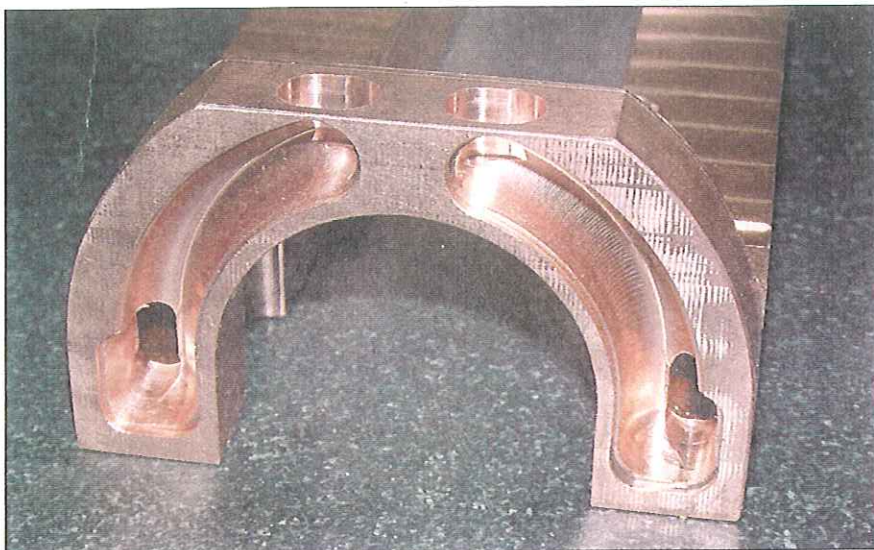
Machined induction coil component showing cooling passages.
