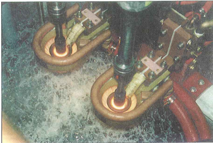
Quenching induction heated parts in a dual scanner set up.
