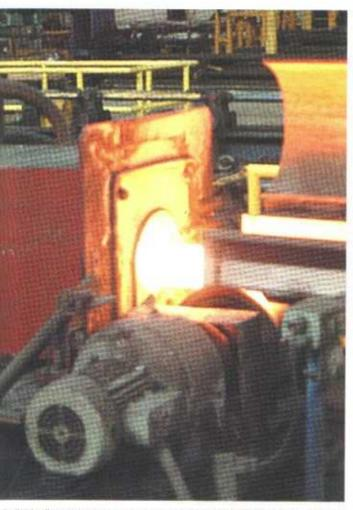
Individually powered control zones enable the Ajax TOCCO Magnethermic induction heating system to remove the end to end temperature taper in seamless tube prior to stretch reduction. Other benefits of induction heating include reduced floor space, cooler working environment, dramatic scale reduction and improved product.
