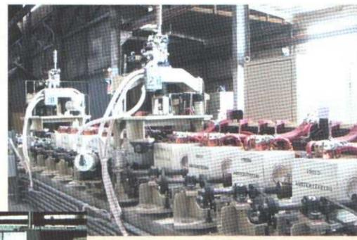
Ajax TOCCO Magnethermic pipe heating lines are known industry wide for producing superior metallurgical and physical properties in the final product. These benefits are achieved with the fast heating rates and temperature control possible only with induction heating.
