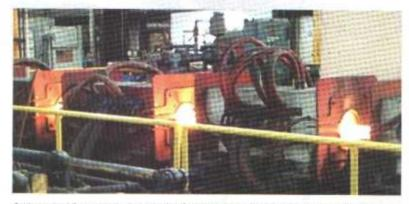
As is typical for most in-line production systems with frequent up and down times, operating costs are reduced since no holding temperatures are required during idle time.
