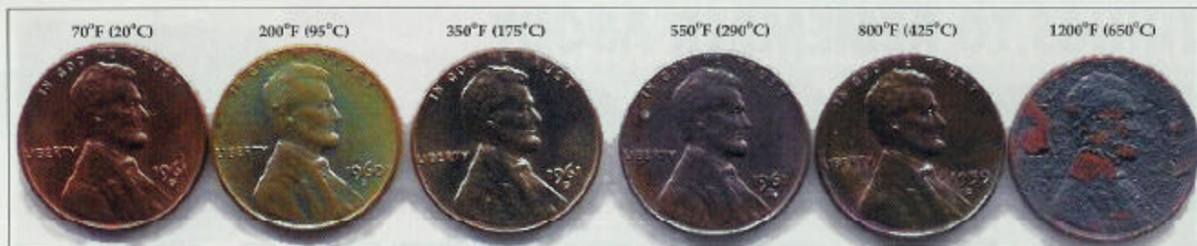
Fig. 2 — Pennies discolor at various temperatures. Copper coil discoloration can be a diagnostic tool to ID problem areas.
