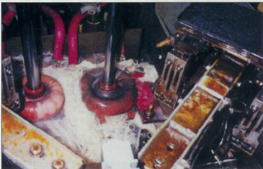
Fig. 3 — Quenchant is diverted by simple cones, preventing overspray.
